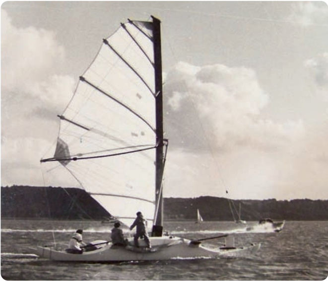
GODIVA with its wishbone rig. This graceful development was thanks to Denis Gliksman.
